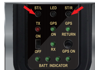
If boat steer to right without steering input, press ST/L button to adjust boat run straightly. If boat steer to left without steering input, press ST/R button to adjust boat run straightly.
