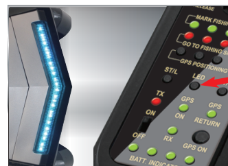
Press LED button one time, the night navigation light turns on, press the button again, the night navigation light turns off
