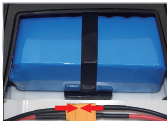
Fix battery with velcro strap, Connect battery with receiver plug inside boat.
